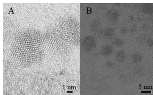
**Figure 1.** TEM images of A) polymer-coated, PEGylated CdSe QDs and B) peptide-coated, PEGylated InAs QD cores. Samples were imaged on glow-discharged, ultrathin carbon Type A TEM grids using a CM20-FEG microscope operating at 200 kV. TEM imaging revealed all QDs to be well dispersed and crystalline.
