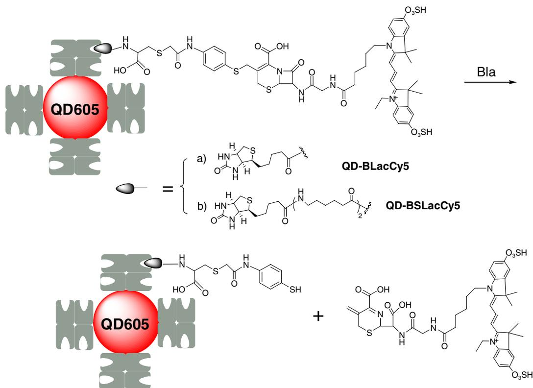
Fig. 1. Schematic presentation of the design of the QDot-based nanosensors for detecting Bla. The Bla substrate is labeled with the FRET acceptor Cy5, and immobilized to QDots via the biotin and streptavidin binding. Bla activity cleaves the lactam ring and releases Cy5 to restore the QDot fluorescence emission.
